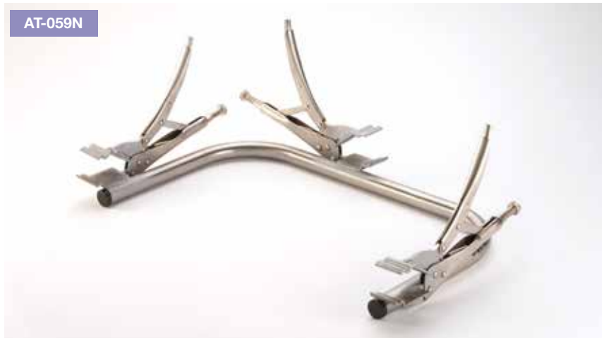
AT-059N: Holding cable clamp. This clamp should be used for cables under tension, keeping the conductors from springing the mold open or being pulled out during welding reaction.
